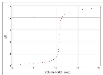
Figure 3 Acid-base titration for sodium hydroxide and hydrochloric acid
