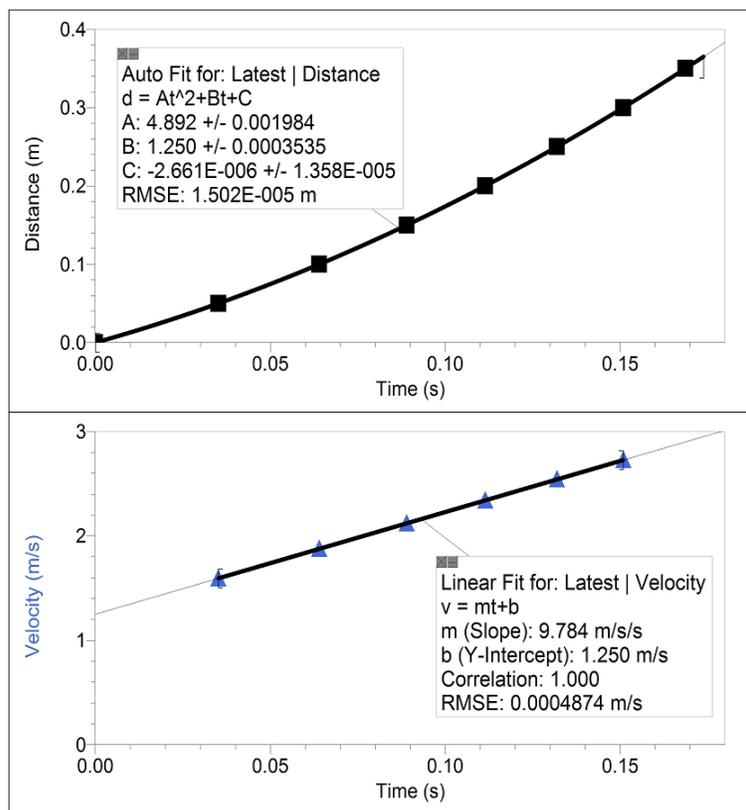
Figure 1 Distance and velocity of Picket Fence in free fall
