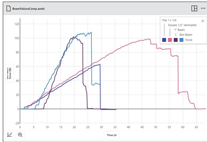
Figure 2 Student results will vary depending on adhesives, materials, and construction techniques used.
