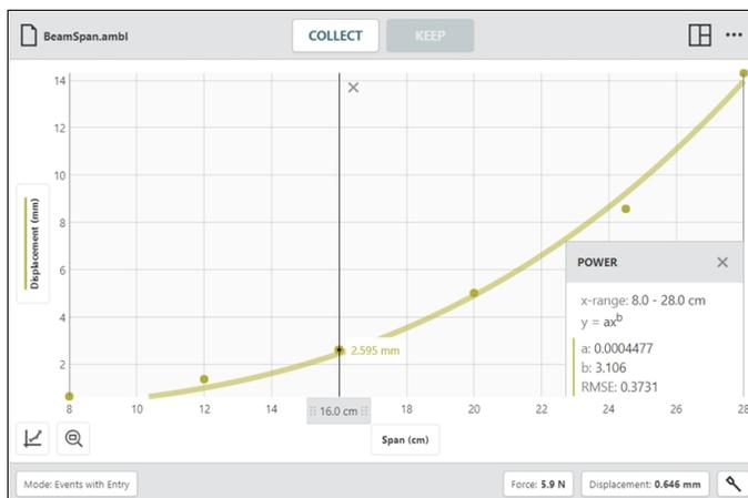
*Figure 4 Span versus displacement*
