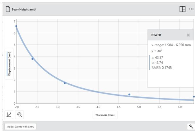
*Figure 3 Beam height versus displacement*
