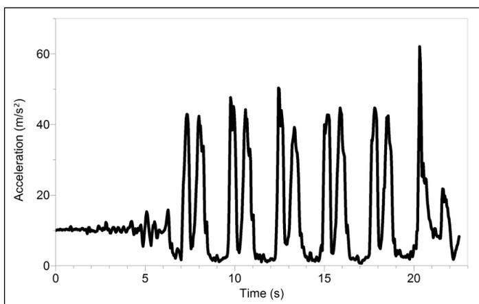
*Figure 2 Acceleration data from a BMX bike on a half-pipe*
