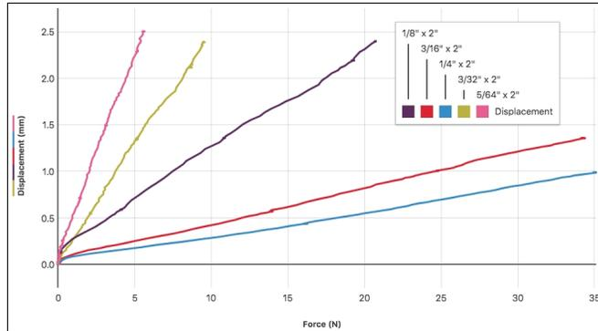
Figure 1 Five data sets of displacement versus force
