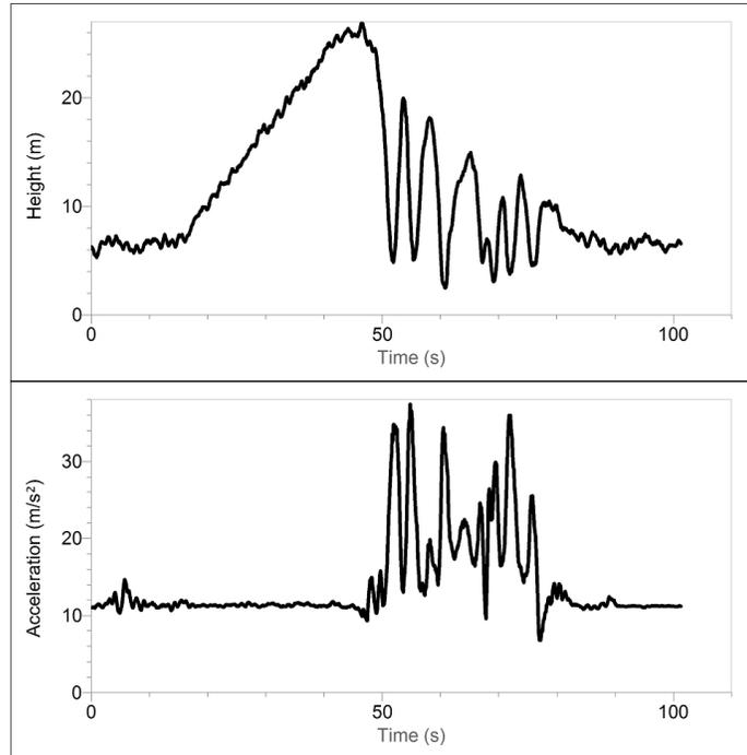
Figure 3 Acceleration data<sup>2</sup> from the Vortex, a stand-up roller coaster
