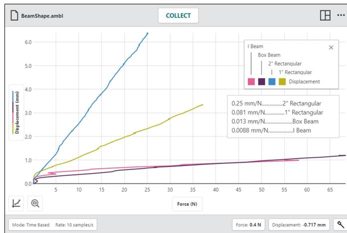
*Figure 1 The beams are tested through their elastic region so that the slope represents their "spring constant." Notice that the plots for the Box Beam and the I Beam have very similar slopes.*
