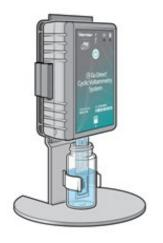
Press the power button to turn on the Go Direct Cyclic Voltammetry System.
