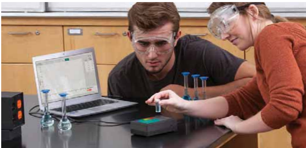
Create an absorbance vs. concentration graph to study Beer's law using copper sulfate.
