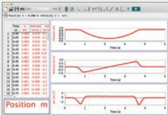
Plot position, velocity, and acceleration data from a Motion Encoder Cart.
