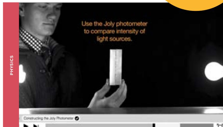
Students measure the total power output of the sun by comparing the intensity of the sun's light at Earth's surface to the intensity of a known source of light.
