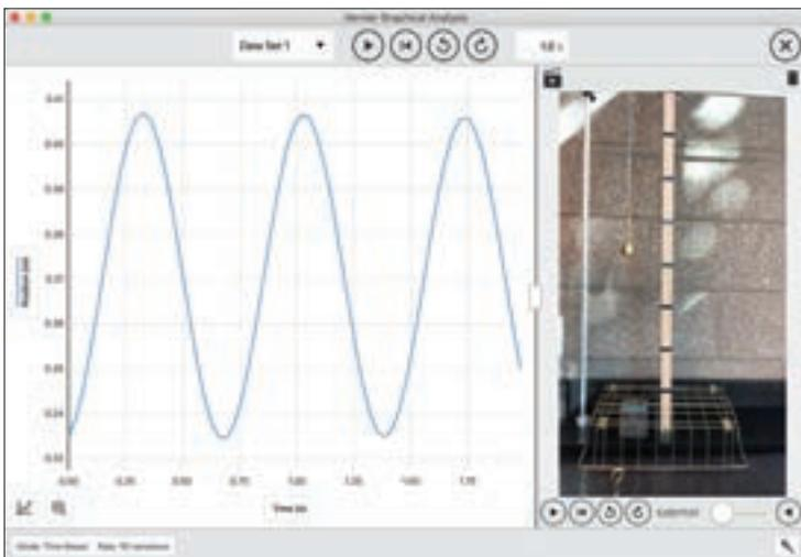
Videos synchronized with sensor data help students understand experiment phenomena such as simple harmonic motion.
