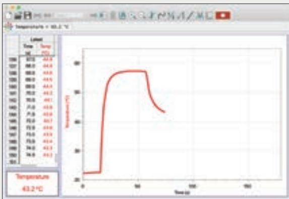
After you click Collect, Logger Pro 3 draws the graph in real time, and the data table and digital meter update continuously.
