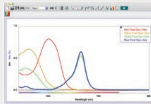
Collect absorbance data from Vernier spectrometers, including our Go Direct SpectroVis Plus and Vernier UV-VIS Spectrophotometers.
