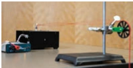
Students explore waves on a string that is fixed at both ends, create harmonics, and relate string tension and wave speed.
