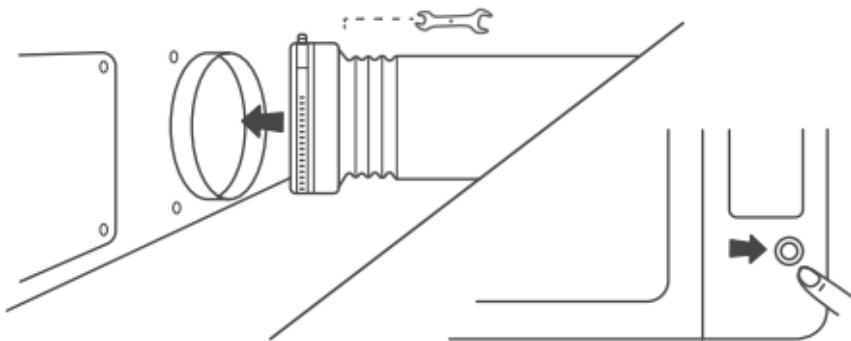
3. Turn on the machine by pressing the power button. The first startup may take up to two minutes.
