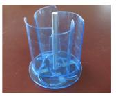
2. Insert the aluminium rotor into the lower blade plate. The rotor can be configured in sets of two to four blades. Use colored markings on the lower and upper blade plate to ensure the blades are in the right positions for each configuration.
