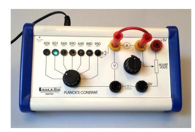
This apparatus provides an array of clear envelope LEDs with peak emission wavelengths in the range 464 to 940nm. The controls allow each LED to be selected in turn and the applied voltage varied so that its electrical characteristics may be investigated. With some simple calculations, an estimate of Planck's constant may be made, the accepted value being:
