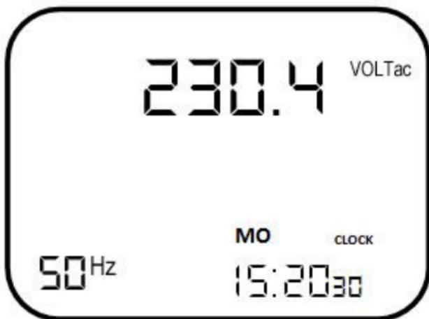
Press the MODE button to switch to the CURRENT range. Here you can check the load current in amps, power factor, weekday and the current time.
