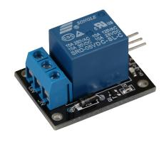
With the relay you can switch higher voltages by using a 5V output. This module can be soldered solidly or can be plugged on a breadboard.
