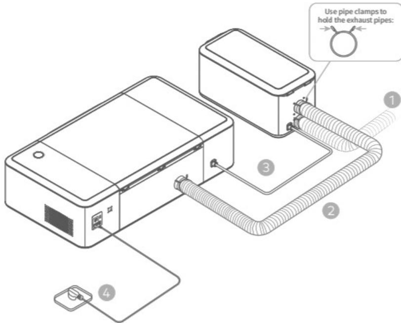
1. Plug the 2m exhaust pipe into the purifier and lead the pipe to the window.
