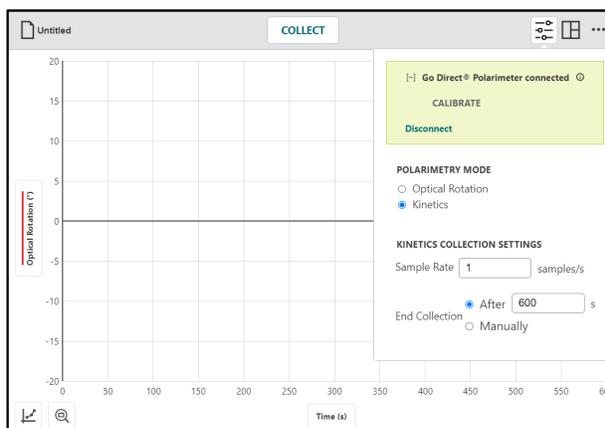
**NOTE:** Collecting more than 10,000 points can impact performance of the app. You can improve performance of the application by turning off the Illumination and Angle sensor channels when connecting your instrument.
