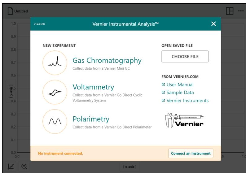
When Instrumental Analysis is launched, the New Experiment box displays the experiment options available in the Instrumental Analysis app. The options are specific to the instrument you are using and provide access to instrument configuration, data-collection settings, and data displays optimized for that instrument. From here, you can also open saved experiments, access online tutorials, and view sample data.
