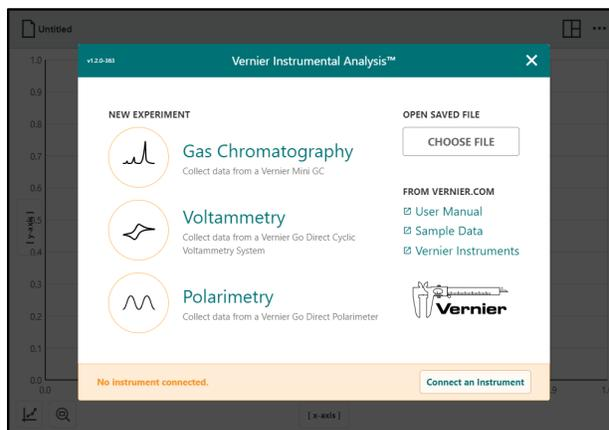
2. If required, connect your instrument to AC power. Turn the instrument on (the Bluetooth LED will flash red). Click or tap **Connect an Instrument** to access the Instruments connection screen.
