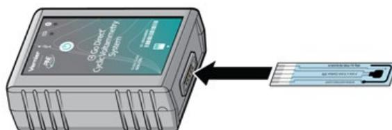
Fill the scintillation vial about halfway full (~10 mL) with your sample. Insert the scintillation vial into the clip on the stand. Carefully guide the Go Direct Cyclic Voltammetry System with the SPE attached downward into the vial and snap the instrument into place.
