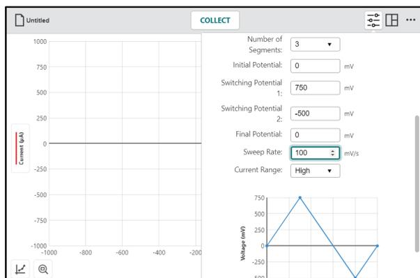
A graph of the voltage (mV) vs. time (s) waveform that will be applied during data collection is shown at that bottom of the Voltametric Settings dialog.
