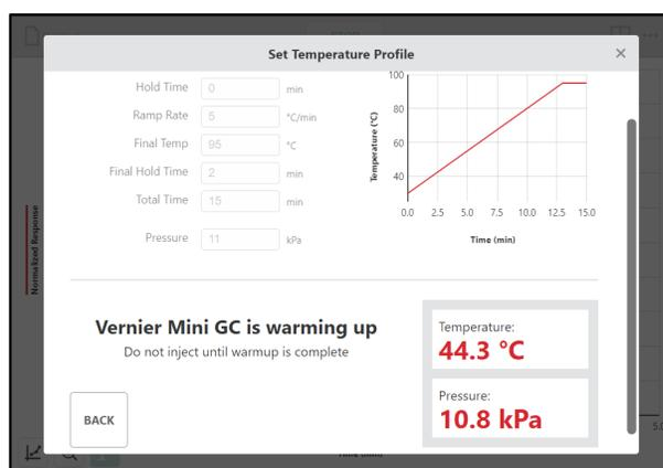
The dialog displays a warmup is complete message when the GC is ready for injection.
