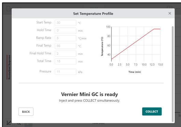
Simultaneously depress the syringe plunger and click or tap **COLLECT**.
