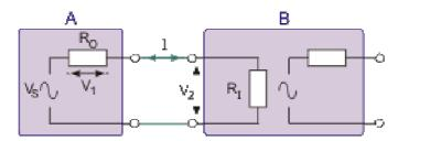
The diagram shows two subsystems, **A** and **B**. Our design aim is to pass on as much of the voltage  $V_S$  as possible. In other words, we want  $V_2$ , the voltage 'seen' by **B**, to be as close as possible to  $V_S$ , the voltage generated by **A**.
