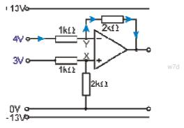
Earlier we pointed out that the ideal op-amp has infinite input impedance, and so draws no current from its input source. We will assume that this op-amp is ideal!
