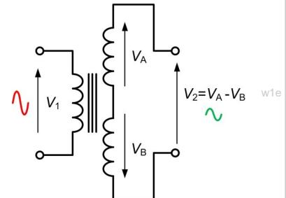
The LVDT requires an AC input, of a few volts amplitude with a frequency usually of a few kilohertz. This generates an alternating magnetic field, which is intensified in the core. This, in turn, induces an alternating voltage in the secondary coils. The greater the overlap of the core and the secondary coil, the greater the voltage induced.
