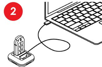
Plug the Micro USB cable into the charger. Plug the other end into a power source, like a computer or external power source.
