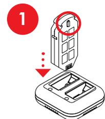
Insert the battery into the charger, with the **tab** facing towards the middle of the charger.
