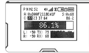
Your connection status screen will display your signal strength. Use **(S)** and **(P)** to change display mode screens in the remote control state.
