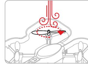
Blow on the attached propeller. Look for difficulty rotating or wobbling during rotation.
