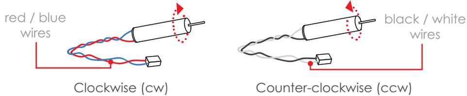
You can see the color of the motor wires by checking **underneath the arms of the drone frame**.
