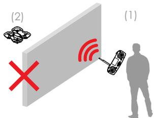
To maximize signal strength and safety, maintain line of sight between yourself/the controller (1) and the drone (2).
