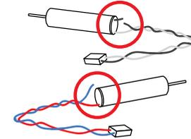
Check for breakages in the wiring. This can happen from hard crashes.
