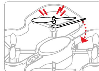
Make sure that the replacement propeller's rotation is correct, and perform a quick flight check.
