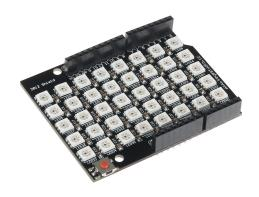
The LEDs are connected in a continuous series. Each LED can be individually receive a color value by digital control. This makes it possible to generate complex color light shows. Each LED can display up to 16 million colors (256 brightness levels/color).
